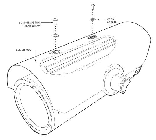
Figure 12. Install the Sun Shroud
